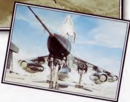
▲ The B-58 was a technological wonder, with blistering performance. Its operational flexibility was limited, however, to the strategic role by its unusual combined fuel- and weapon-pod concept.
